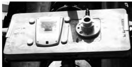
PV cell solar meter (left), thermocouple pyranometer (right).
